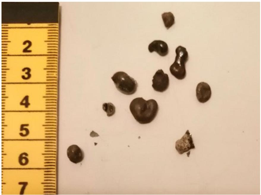
Large globules with an uneven surface - partly magnetic
