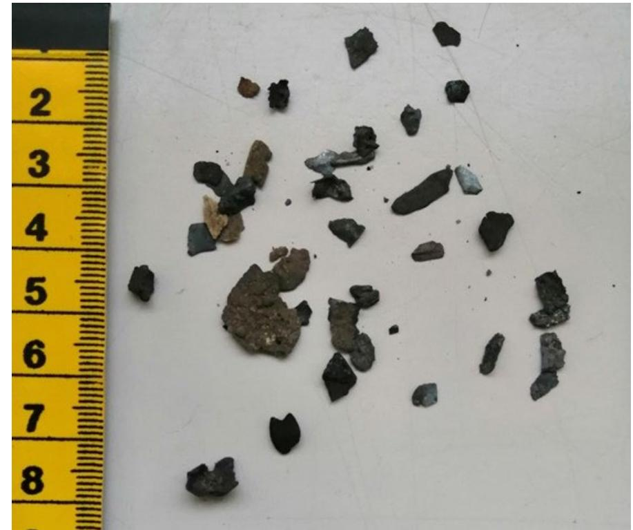
Large scales with an uneven surface – partly magnetic
