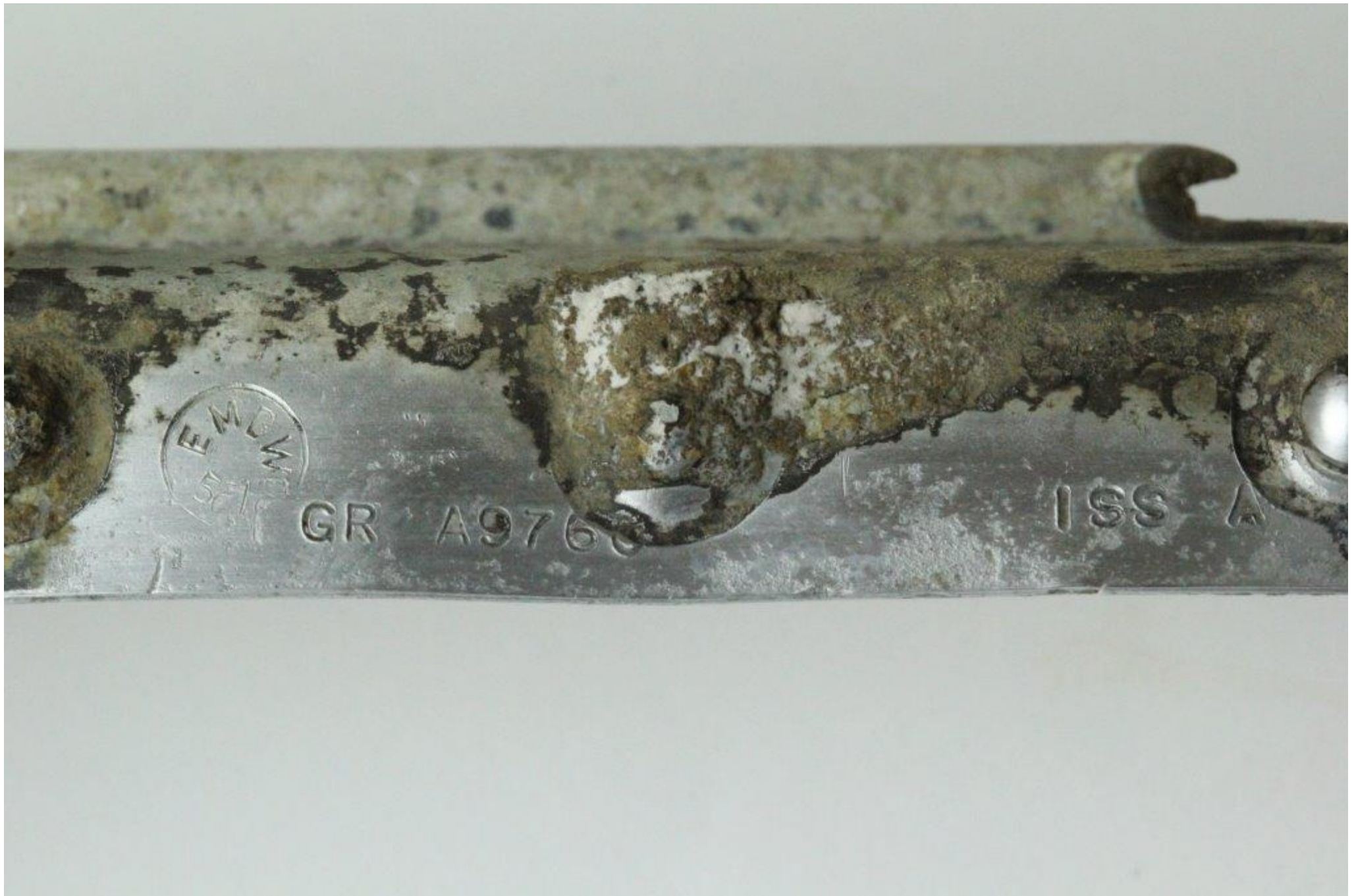
Aluminium wreckage with part numbers and inspection stamps.
