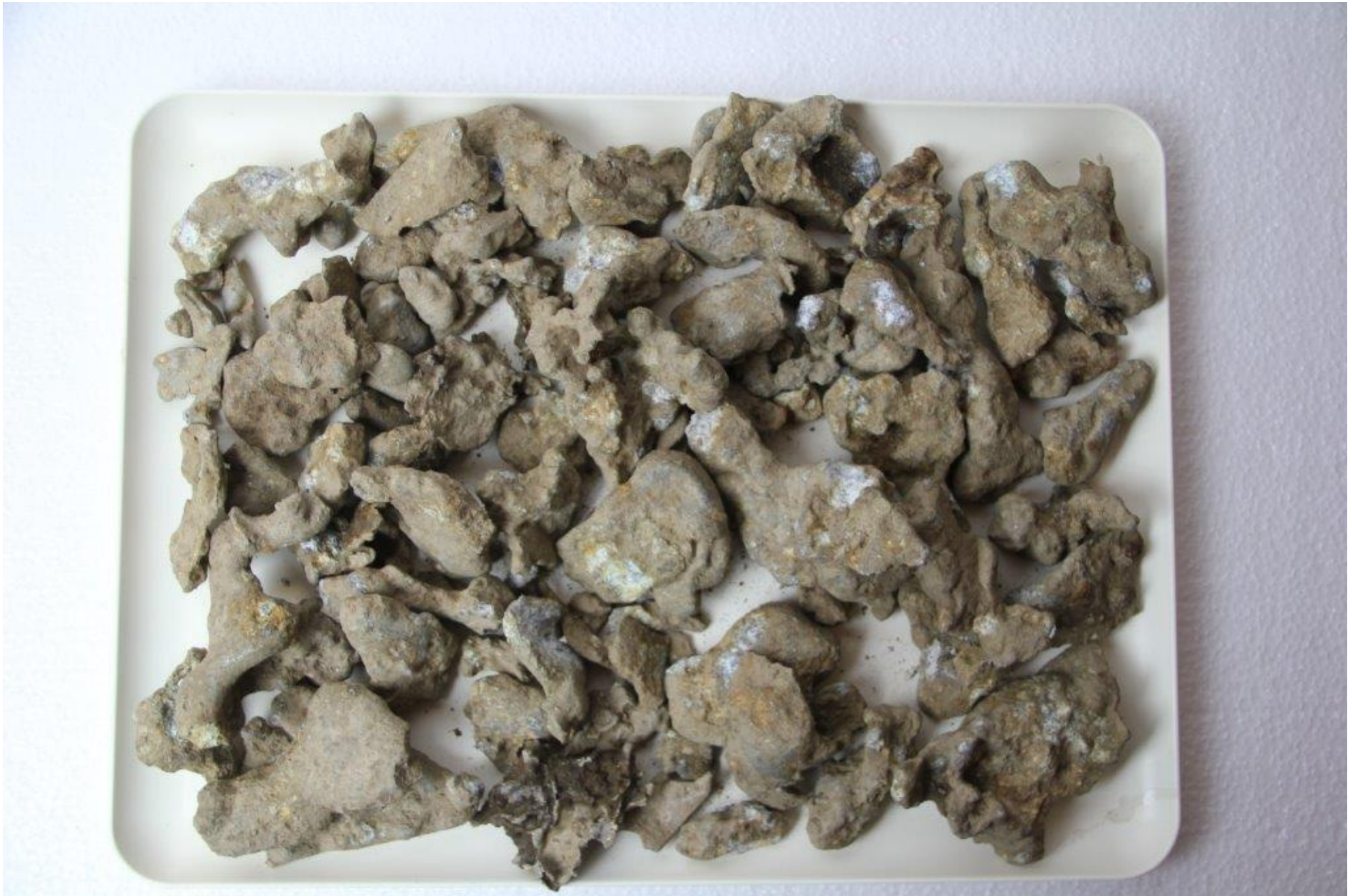
Debris field 1: Molten aluminium from the aircraft fire (100 pieces, 3 kg).
